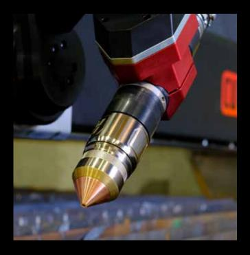
Utilising the Hypertherm XPR plasma system, cut angles of up to  $\pm 50^{\circ}$  can be achieved with unlimited winding.
