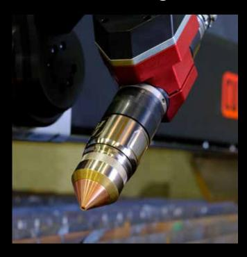
Utilising Plazmax's very own in house designed and manufactured compact CNC Bevel Head, cut angles of up to  $\pm 50^{\circ}$  can be achieved with ease.
